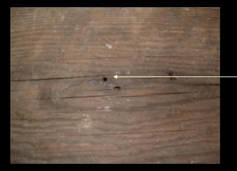
THERE MAY BE BROKEN NAILS IN THE WOOD AND THEY WOULD DAMAGE THE PLANER KNIVES
